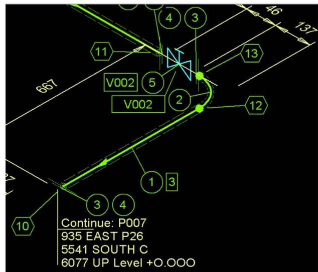
Pic. 12. Example of an isometric drawing
