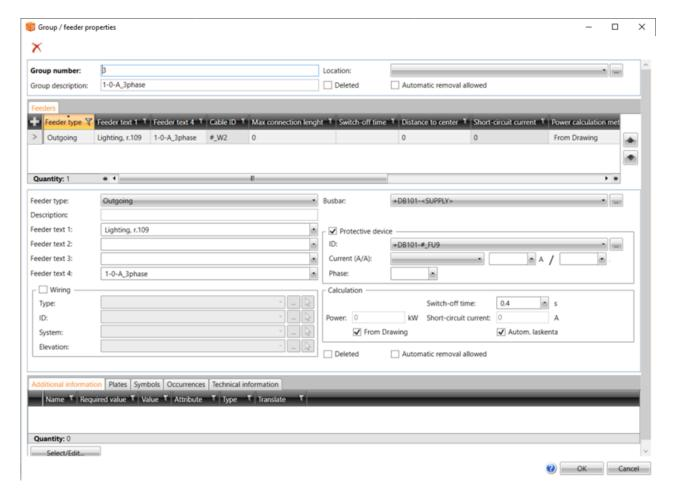
Furthermore, protective devices can be added for feeders. This means that the protective device will create a device in the database, and an occurrence of the device can then be inserted into the schema. This allows presenting devices related to feeders in separate documents, in addition to which the database structure will be more realistic.
