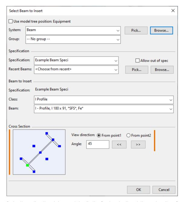
During the routing, there is improved visualization for changing the rotation angle or the reference point.
