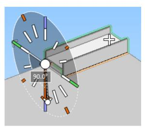
In addition, the beam tools now include a **Join** command for joining two beam parts that have a
