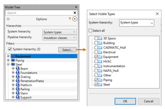
When the required object or group is found, the user can see its current check-out status from the tree and perform a check-out or check-in as necessary. Selecting an item from the model tree (or from a work view) shows that entity's properties in the new **Properties** pane. **You can copy a property value from the Properties pane with Ctrl+C.**
