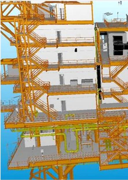
*Val d'Agri plant example: the model was created in PDS by Italia Progetti srl and converted into eBrowser*
